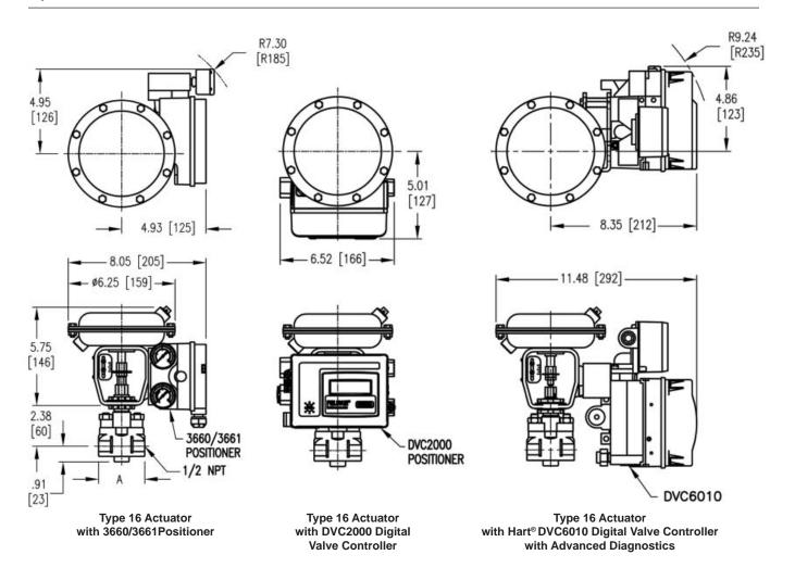
Figure 5. Dimensions - inches [millimeters]
